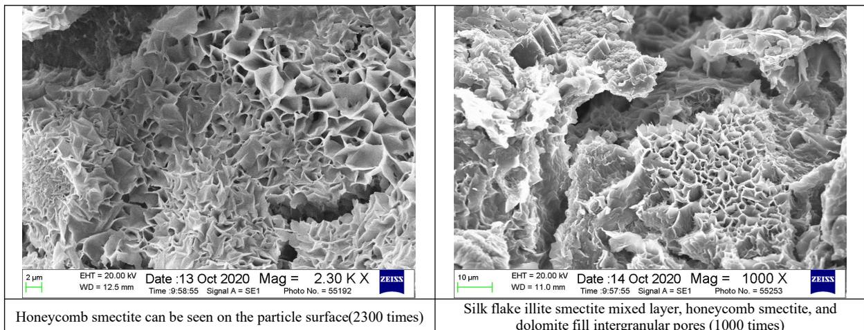
**Figure 9:** Water sensitivity mechanism
