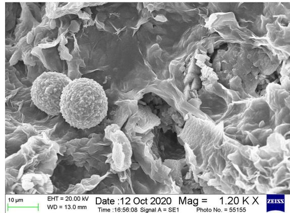
Intergranular pores filled with spherical pyrite, silk flake illite, smectite mixed layer, and kaolinite (1200 times)
