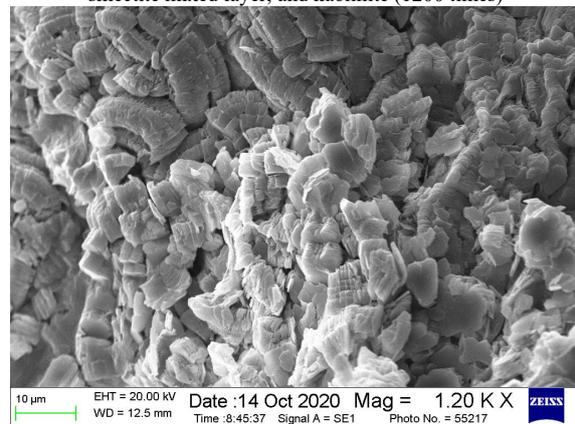
The mixed layer of scaly kaolinite, illite, and smectite fills intergranular pores, and the stone fills intergranular pores (1200 times)
