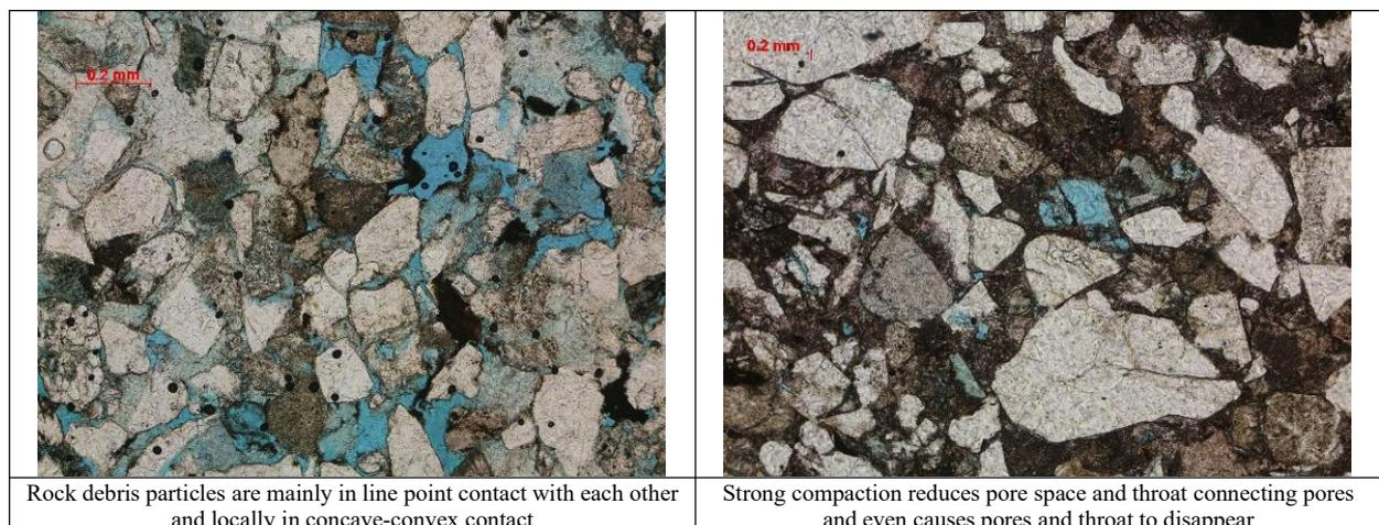
**Figure 11:** Stress sensitivity mechanism
