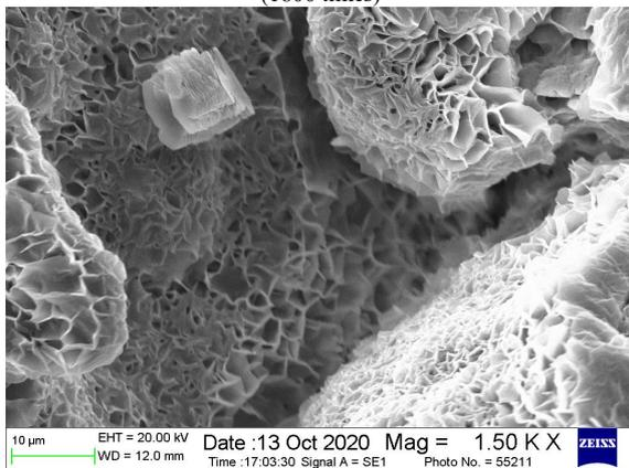
Honeycomb smectite and scaly kaolinite fill intergranular pores (1500 times)
