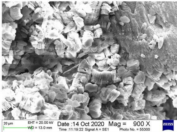
Filling intergranular pores with scaly kaolinite (900 times)
