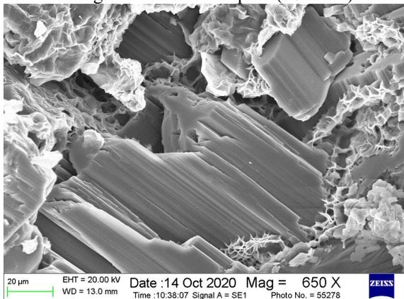
Feldspar dissolution, silk flocculent smectite, and illite smectite mixed layer filling intergranular pores (650 times)
