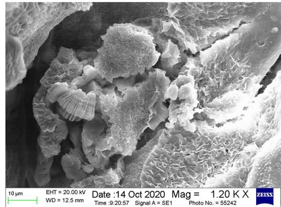
Silk flocculent smectite, illite smectite mixed layer, and book leaf kaolinite fill intergranular pores (1200 times)
