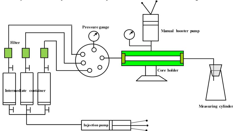
**Figure 2:** Schematic diagram of sensitivity test
