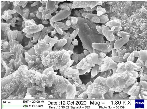
Authigenic quartz, halite, illite, and kaolinite fill intergranular pores (1800 times)
