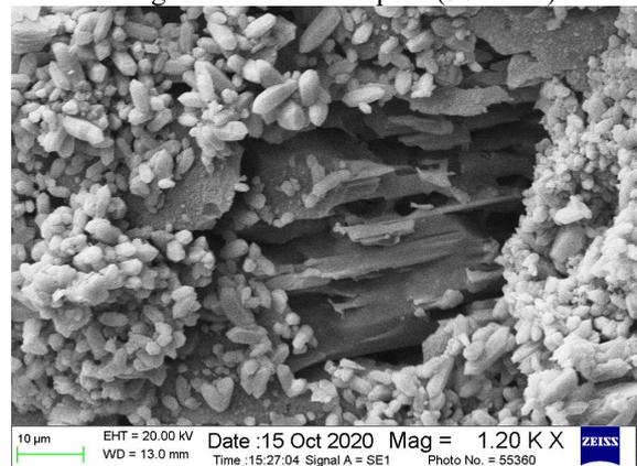
Feldspar leaching corrosion hole, with authigenic quartz around (1200 times)
